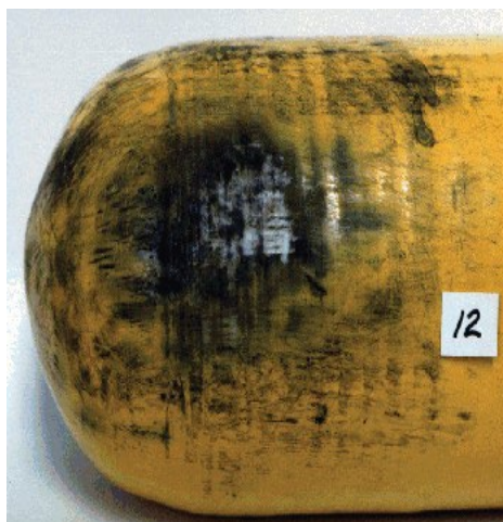
Figure 6: Heat and Fire Damage
