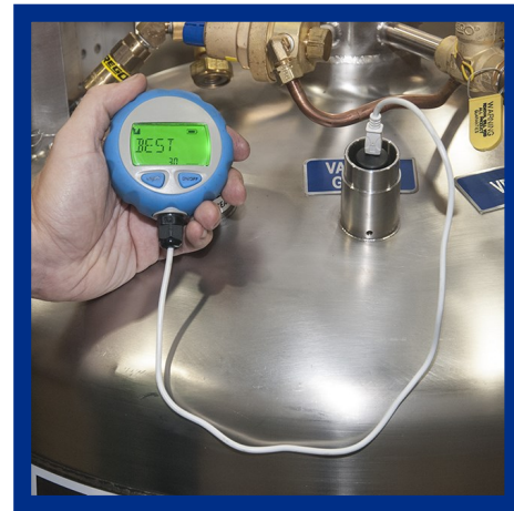
The vacuum gauge and reader gives our customers the ability to perform a diagnostic test on their cylinders prior to sending them to be repaired.
